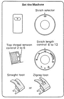
results are NOTE: Best sewing obtained with the straight stitch foot, but the zigzag foot will also provide acceptable results.
